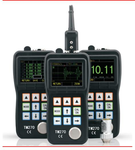
The handheld TM270 series ultrasonic thickness gage uses dual element transducers for corrosion applications. It offers many basic features such as Min/Max Mode that measures and recalls the minimum thickness at a fast 20 readings per second, Freeze Mode to instantly capture critical thickness, and Zero Compensation, A-scan display for echo-echo measurement.
